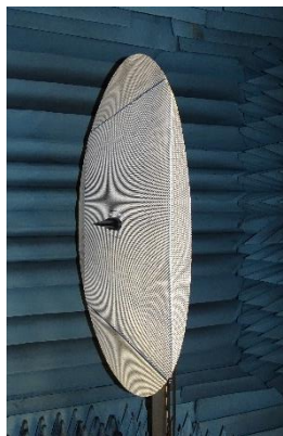
antenna sample measured on Ø52in (1.3m) ground plane
